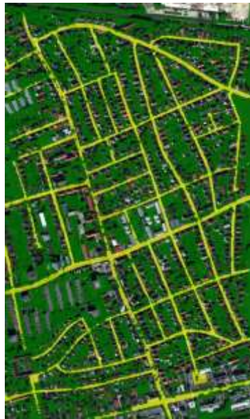
Figure 3: Based on the NDVI, a vegetation mask is applied [Tama Group Ruleware]
