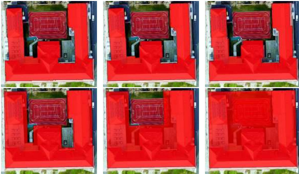
Fig. 7: Generalization of building outlines for different degrees of abstraction
