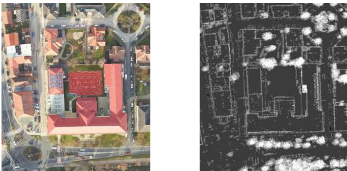
Fig. 1: Example of an RGB image (left) and LiDAR information (right) displaying the number of returns (the brighter the more returns)
