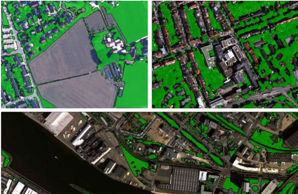
Fig. 2: Vegetation extracted by Tama ruleware on eCognition for the three different test sites.
